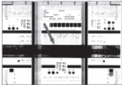
19. The copy is foggy (cross-feeding direction).
