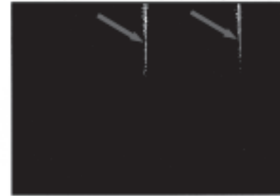
16. The copy has displaced registration (leading edge, excessive margin).
