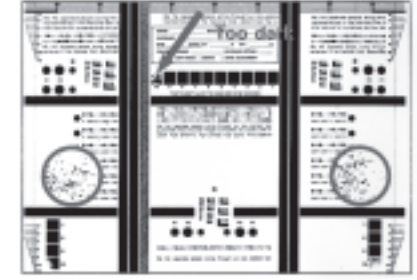
12. The copy has white strips (cross-feeding direction).
